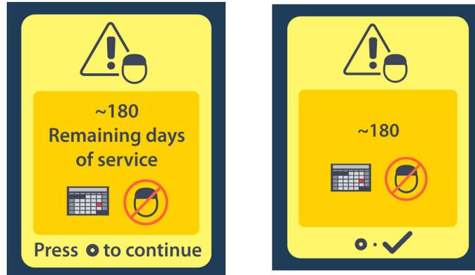
Press [stimulator icon] to clear the message. The message will reappear approximately weekly until the end of the non-rechargeable Stimulator's programmed period is reached. When the end of its programmed period is reached, the Remote Control will display the following on-screen message.
