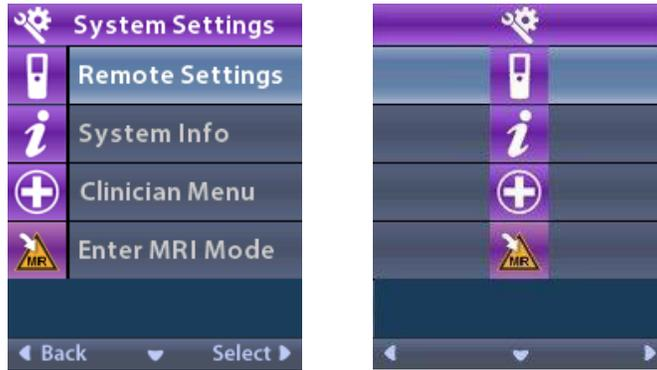
**Note:** When the Remote Control is linked to a Vercise Gevia rechargeable Stimulator, the Enter/Exit MRI Mode icon will appear on the System Setting screen. Refer to the MRI Mode section for information on the Enter/Exit MRI Mode feature.
