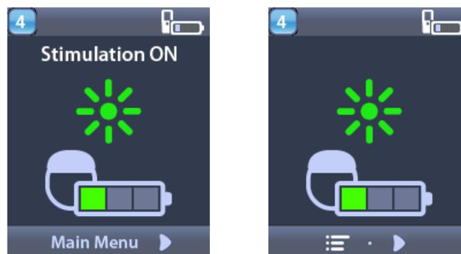
**Note:** *When the Remote Control connects to a rechargeable Stimulator, it will display the current battery level of the Stimulator on the Home screen.*
