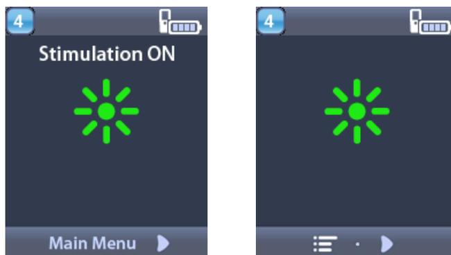
**Note:** When the Remote Control connects to a non-rechargeable Stimulator, the battery level of the Stimulator will not be displayed on the screen.
